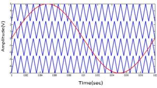
Fig 3.2 Carrier arrangement for PDPWM
