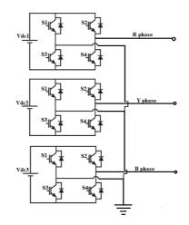
Fig 2.2 Cascaded 13-level multilevel inverter
