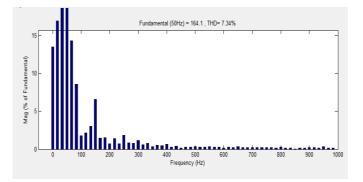
Fig 4.2 THD Calculation for thirteen levels
