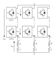
Fig 1.1 General configuration of the proposed three phase cascaded multilevel inverter
